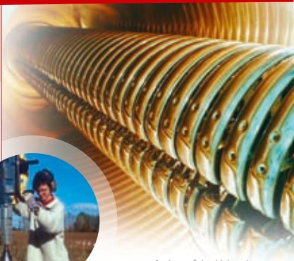
A view of the high voltage generator of the ^{14}\text{C} -accelerator.
